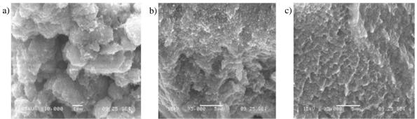
FIGURE 2. SEM images of (a) TiO<sub>2</sub> (b) TiO<sub>2</sub>-GO and (c) TiO<sub>2</sub>-rGO surfaces.
