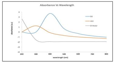
FIGURE 3. Uv-Vis graph of GO and rGO solution.
